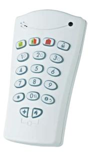
WK-141 is a portable, wireless, two-way keypad for DSC WP. It enables easy arming and disarming of the alarm system and initiation of emergency, fire and panic alarms. It also controls programmable outputs (PGM) and X-10 devices from anywhere in the premises. Two-way communication with the control panel provides homeowners with visual indication of successful command execution and system status.
