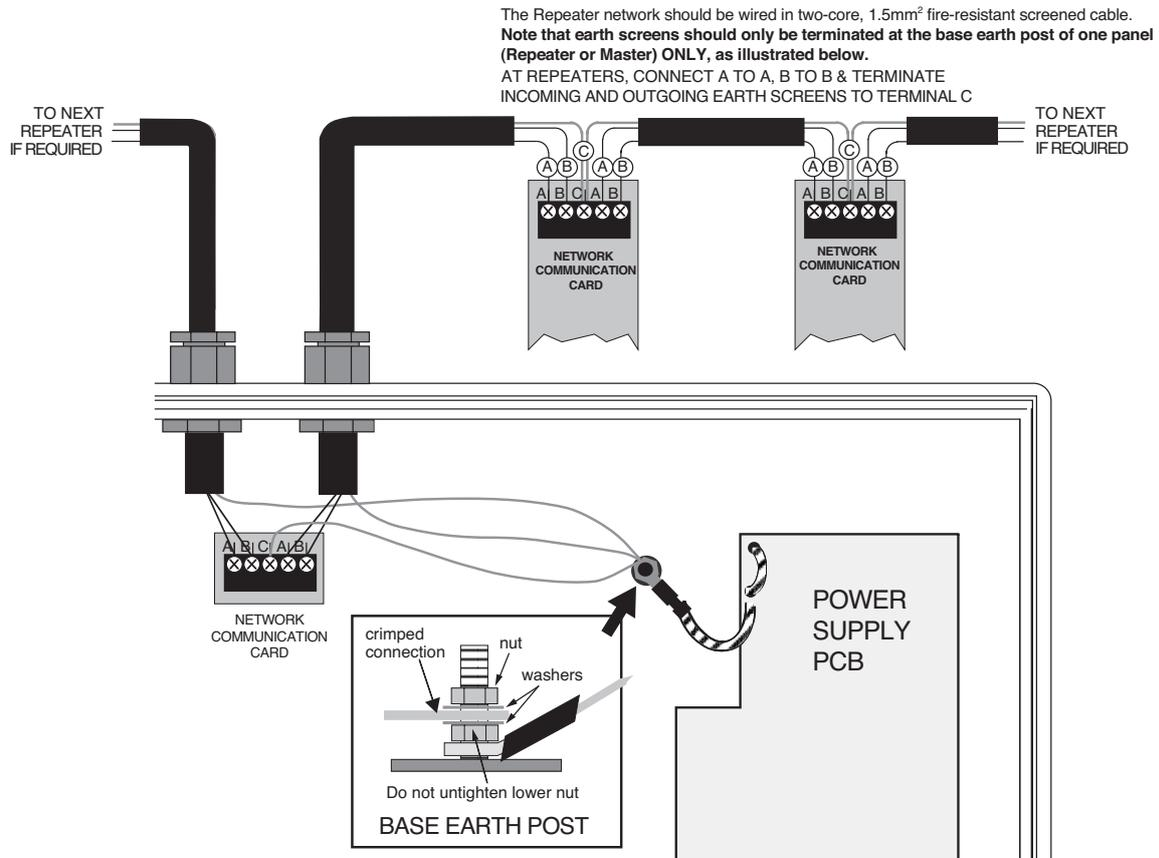
Fig. 7 : A typical XFP Repeater network
