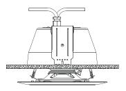
**12)** With the speaker in this position connect the 3 wires hanging from the termination plate on to the speaker using the spade terminals provided.
