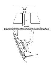
10) The fire dome should be firmly secured into the ceiling.
