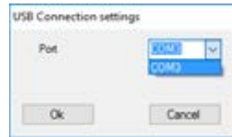
PICTURE 2. Selecting the COM port for connecting the receiver to the computer
