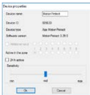
PICTURE 5. The sensor's properties' menu makes it possible to register the sensor in the zone
